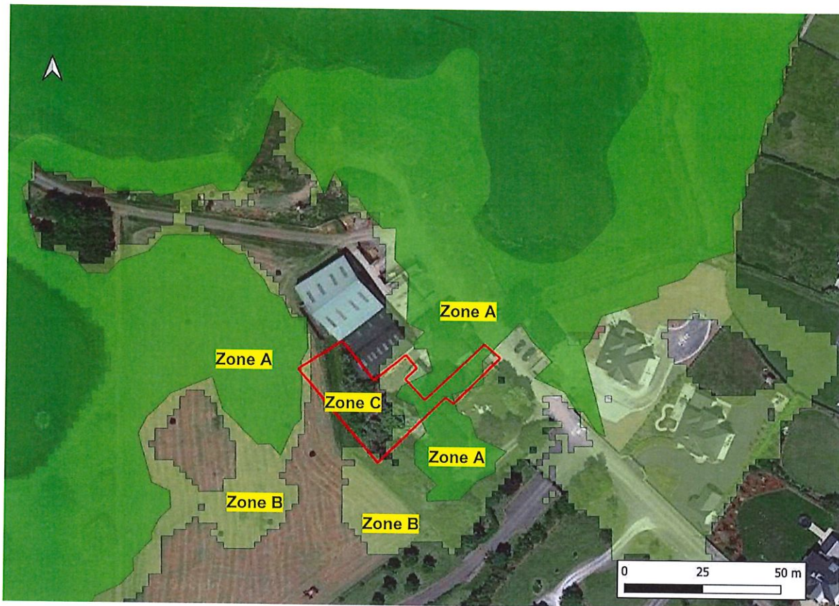
Figure 3-3 Coastal Flood Risk Mapping in the vicinity of the development at Renville West Oranmore (200 and 1000year tidal flood extents from the ICPSS and OPW Floodinfo mapping)
